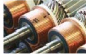
We produce coils in round wire or flat wire design and rely on high quality insulating materials and vacuum impregnation.
