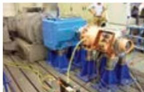
We have over six test facilities for load tests up to 55,000 Nm and we use a water recooling system for motors and converters.
